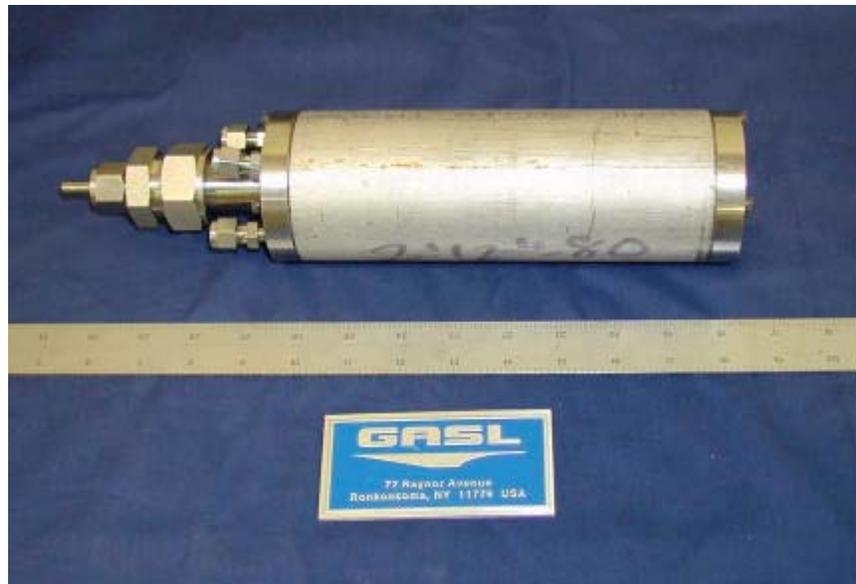
Figure 2: Photograph of the ethylene/air combustor used in this work (scale in inches).
