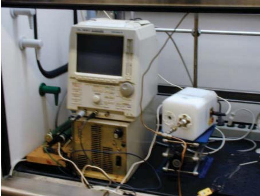
Figure 6: Fan-type plasma reactor (white box on right) shown with Japan-Inter uHV-10 AC power source and Yokogawa digital oscilloscope DL 1520, as used in experiments conducted at the University of Connecticut.
