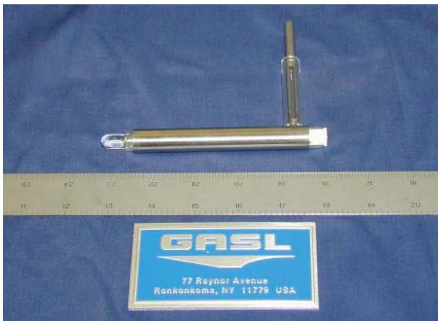
Figure 4: All-quartz tubular reactor, shown with Inconel electrodes (scale in inches).
