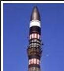
The U.S. Peacekeeper ICBM (formerly MX), the most modern ICBM used by the United States during the 1990s. Its design combines advanced technology in fuels, guidance, nozzle design, and motor construction with protection against the hostile nuclear environment associated with land-based systems. The Peacekeeper is much larger than Minuteman, over 70 feet long and weighing 198,000 pounds.
