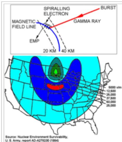
The mechanism for a 400 km high-altitude burst EMP: gamma rays hit the atmosphere between 20-40 km altitude, ejecting electrons which are then deflected sideways by the Earth's magnetic field.
