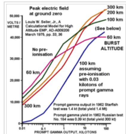
How the peak EMP on the ground varies with the weapon yield and burst altitude. Note that the yield here is the prompt gamma ray output measured in kilotons. This varies from 0.1-0.5% of the total weapon yield, depending on weapon design.
